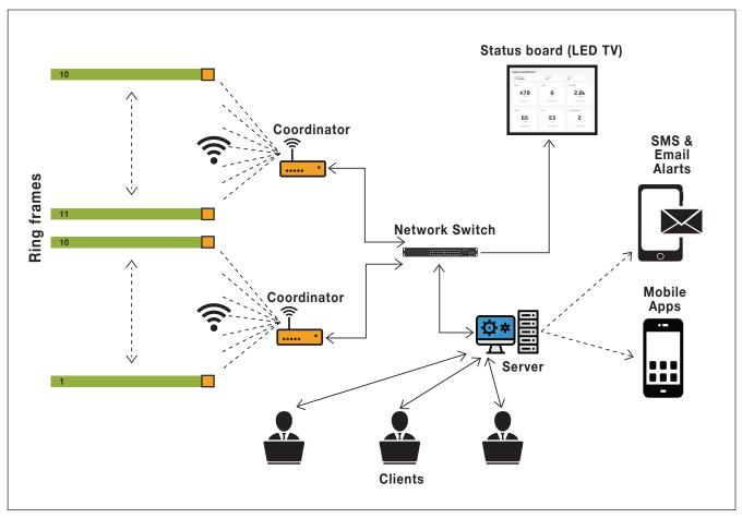
Figure: A macro view of IoT-based production monitoring system
